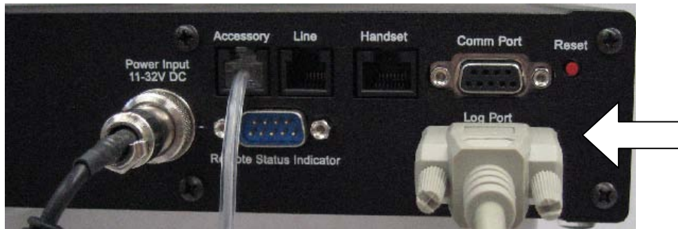
Figure: Serial cable connected to Log Port
