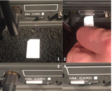
Installing SIM card and engaging the lock
